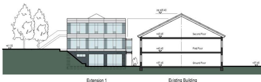
SECTION C - NORTH-EAST ELEVATION EXTENSION 1
